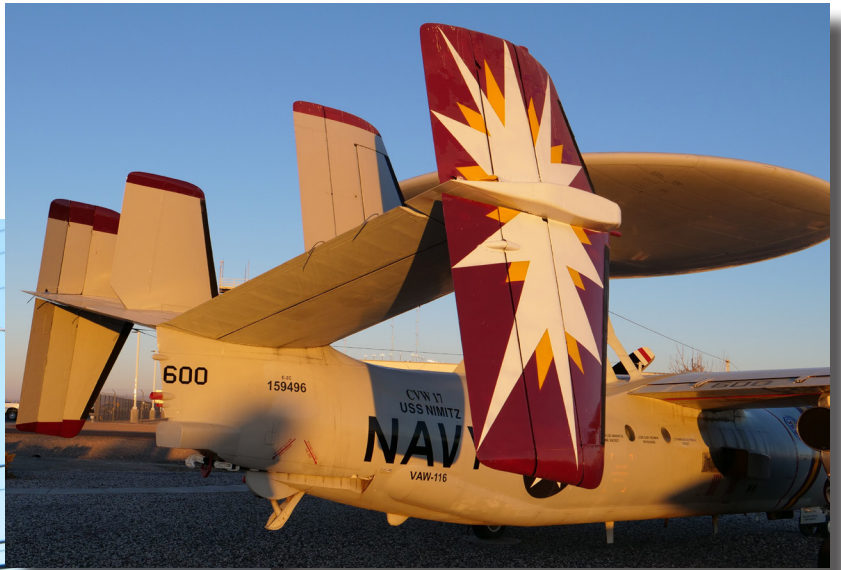
The tail of the E-2C Hawkeye command and control aircraft sports four vertical tails giving it superior yaw control for landing aboard an aircraft carrier.
